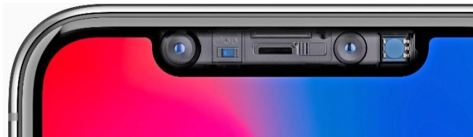
Apple Face ID structured light sensor 940 nm
