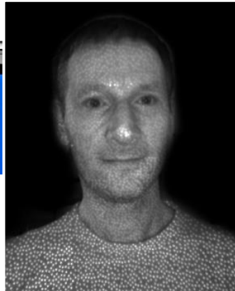
Apple Face ID structured light sensor 940 nm
