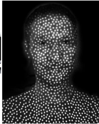
Intel RealSense structured light sensor 850 nm
