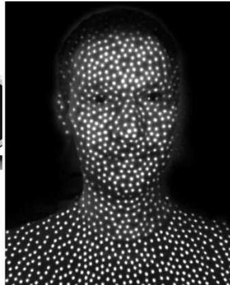
Intel RealSense structured light sensor 850 nm
