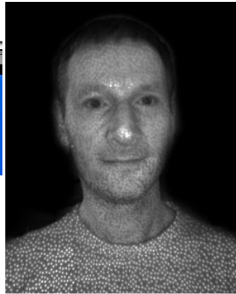
Apple Face ID structured light sensor 940 nm
