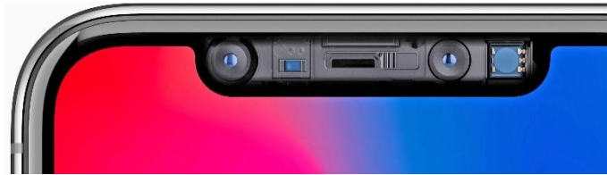
Apple Face ID structured light sensor 940 nm
