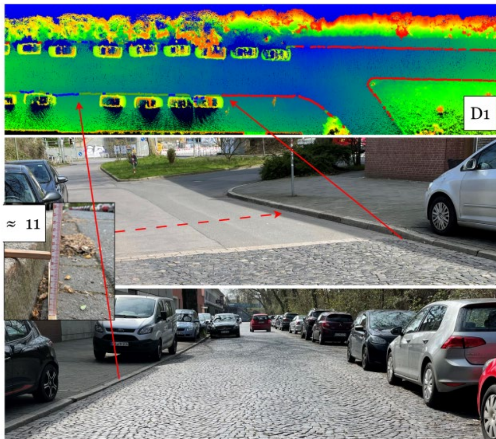
Figure 25: Results for proposed curb detection and height estimation
