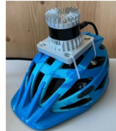
Figure 2: Mounted OS1-128 sensor
