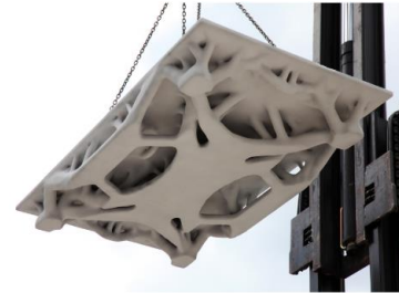
Patricle Bed for Slabs, Credit: Andrei Jipa, DBT, ETH Zürich
