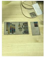
Illustration 11: colors which can be produced with the laser
