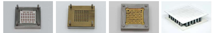
Figure 4. Assembly sequence for TEGs with high aspect ratio thermolegs (here: TEG-1). Bottom ceramic substrate in assembly rig (a), intersecting alignment fixtures (b), inserted thermolegs (1x1x4 mm 3 ) (c), TEG-1 after soldering in reflow oven (d).
